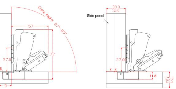
The side panel can be 15-30mm thick, with a maximum thickness of 30mm. The door panel can be 15-25mm thick. If there is another door on the other side, the thickness limit of the door panel is 25mm, and K=5+12 If there is no door on the other side, the thickness of the door panel can be 15-50mm, with K=5+12
